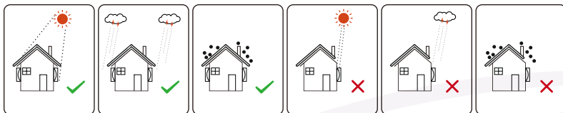
Figure 4-1 Recommended installation location
